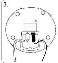
Connect the power supply to the SignWave base and plug adaptor into a 13 Amp mains socket.
