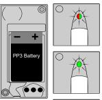
When a battery is first fitted the indicator light will flash red then green a few times.
