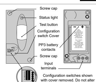
1. Install a 9 volt PP3 alkaline or lithium battery making sure to observe the correct polarity.
