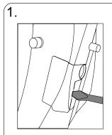
Insert a small flat blade screwdriver into the slot on the front cover.
