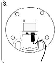
Connect the mains adaptor to the SignWave base and plug adaptor into a 13 Amp mains socket.
