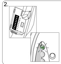
Move the On /Off key to the left using the edge of the front cover.
